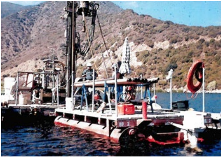
Sampling Barge on Matilija Reservoir, 2001. Drilling, coring, and sample collection was conducted from a barge on the reservoir to obtain subsurface data and sediment samples.
