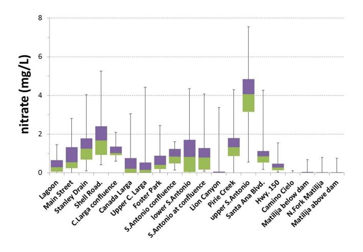
This is a box plot of nitrate in the Ventura watershed. Each box represents the range of the middle half of monthly measurements made by Santa Barbara Channelkeeper (SBCK) since 2001; the line in the middle of the box shows the median – half the measurements were above this value, half below. The end of each bar extending above and below the box shows the highest and lowest monthly concentrations measured.
